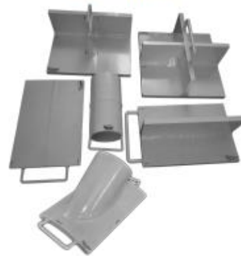
PAUT AND TOFD FLAWED SPECIMENS-PHASED ARRAY ULTRASONIC TESTING
