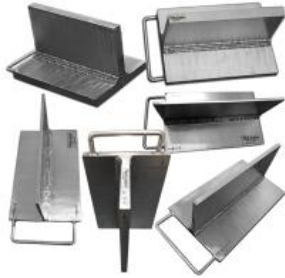
ISO-9712 NDT TRAINING NOZZLE FLAWED SPECIMENS PCN CATEGORY-3.4.1
