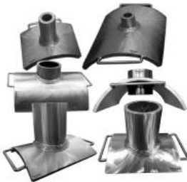
ISO-9712 NDT TRAINING NOZZLE FLAWED SPECIMENS PCN CATEGORY-3.4.1
