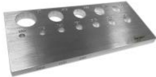
12 HOLE 15 NOTCH GENERAL PURPOSE EDDY CURRENT BOLT HOLE STANDARD BLOCK
