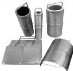
NDT ASME SECTION XI, APPENDIX VII KIT SPECIMEN
