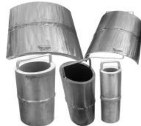
API RP AND API UT FLAW SPECIMEN QUALIFICATION KIT
